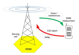
Figure 2. Reporting mechanism between UE and BS.
