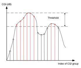
Figure 3. Basic principle of threshold-based CQI reporting.
