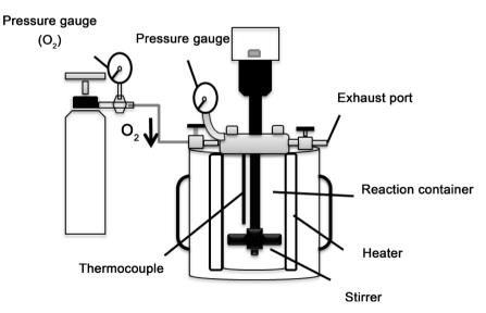
Figure 3. A schematic diagram of autoclave equipment used in the study.
