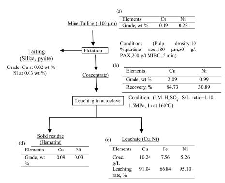
Figure 13. Schematic flowsheet for combined flotation and high pressure leaching for recovery of copper and nickel.
