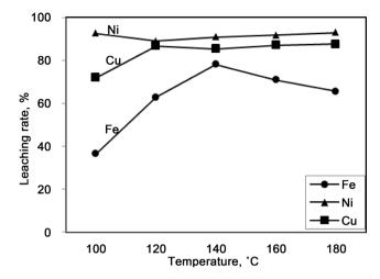
**Figure 9.** Dissolution of flotation concentrate as a function of temperature (1 M  $H_2SO_4$ , 1.5 MPa total pressure, S:L = 1:10 at 400 rpm for 30 min).
