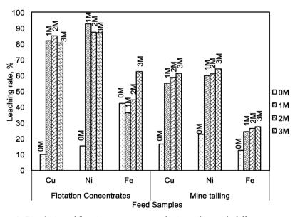
**Figure 8.** Dissolution of flotation concentrate and mine tailing with different concentrations of  $H_2SO_4$  ( $H_2SO_4$ : 0 - 3 M, total pressure 1.5 MPa, S:L = 1:10 at 400 rpm, 140°C temperature for 30 minutes).
