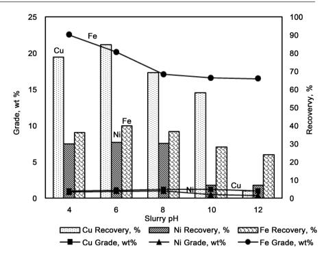
Figure 5. Effect of slurry pH on the recovery of copper and nickel. Flotation conditions: pulp density of 10%, flotation time of 10 min, PAX dosage (collector) of 50 g/t and frother dosage of 200 g/t.
