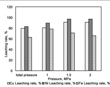
Figure 10. Dissolution of copper and nickel from flotation concentrate as a function of pressure (1 M  $H_2SO_4$ , 1.5 MPa total pressure, S:L = 1:10 at 400 rpm, 140°C temperature for 30 min).
