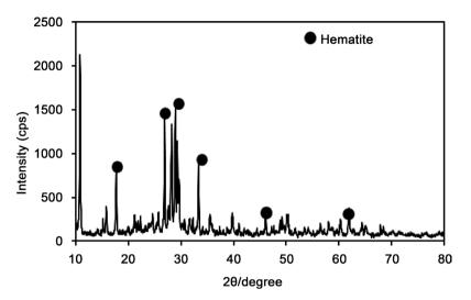
Figure 12. XRD patterns of the froth concentrate from flotation and solid residue from high pressure oxidative leaching.
