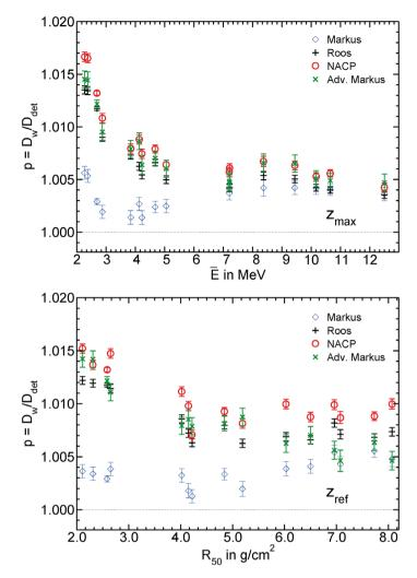
**Figure 3.** Total perturbation correction *p* of parallel-plate chambers as a function of the beam quality specifiers  $\overline{E}_{z,max}$  and  $R_{50}$ . The error bars indicate the statistical uncertainties of the Monte Carlo simulations (1 $\sigma$ ).
