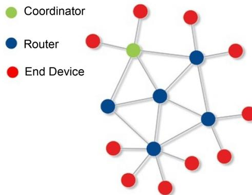
Figure 6. ZigBee network.
