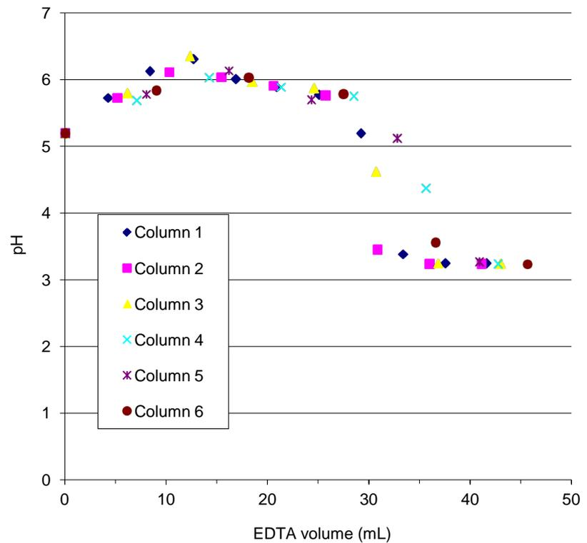
**Figure 3.** pH of EDTA eluent (0.1 mM) measured after its loading in carboxylic calixarene (CC) column as a function of its percolated volume, after U and Am extraction from mineralized urines on CC column at pH 5.2.
