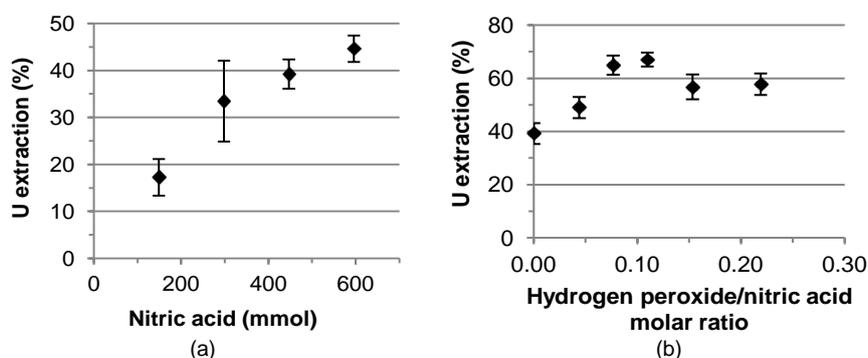
**Figure 2.** Influence of nitric acid quantity (a) or molar ratio of hydrogen peroxide/nitric acid (b) used for the microwave digestion of urine samples on the U extraction yield by the carboxylic calixarene column at pH 5.2. (a) Only nitric acid (10 to 50 mL of 67 wt% nitric acid) was used for the step of microwave digestion. (b) 30 mL of nitric acid (67 wt%) was used in mixture with various volumes of hydrogen peroxide (2 to 10 mL of 30 wt% hydrogen peroxide).
