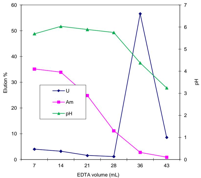
**Figure 4.** Correlation between the pH of EDTA solution (0.1 mM) measured at the bottom of the carboxylic calixarene (CC) column and the elution yields (%) of U and Am as a function of EDTA volume (mL) percolated through the column, after U and Am extraction from mineralized urines on CC column at pH 5.
