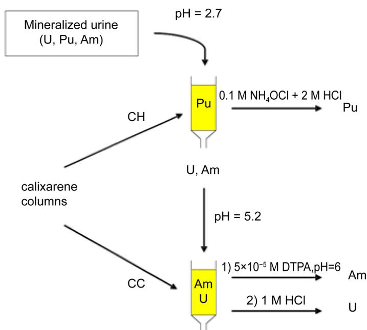
**Figure 1.** Protocol optimized for the separation of U, Pu and Am from mineralized urine using calix[6]arene columns (CH = hydroxamic calixarene column; CC = carboxylic calixarene column).
