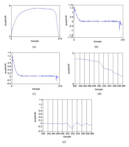
**Figure 5.** a) Experimental signal; b) error signal of the adaptive linear predictor; c) error signal of the IAF; d) zoomed in view of the position of breakdown point in the input signal; e) zoomed in view of the position of the detected breakdown point in the error signal of IAF.
