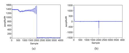
Figure 4. a) Simulated noisy sine wave; b) error signal of the proposed IAF.
