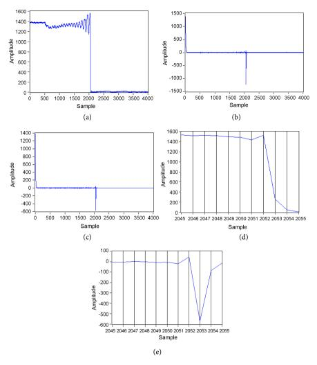
**Figure 3.** a) Simulated faulty powerline signal; b) error signal of the adaptive linear predictor; b) error signal of the IAF; d) zoomed in view of the position of breakdown point in the input signal; e) zoomed in view of the position of the detected breakdown point in the error signal of IAF.
