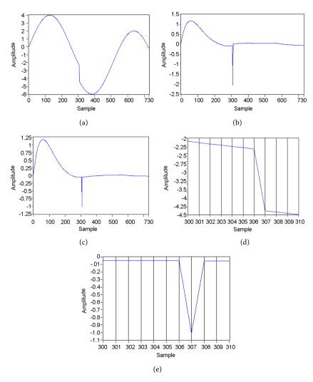
**Figure 2.** a) Simulated sine wave with a breakdown point; b) error signal of the adaptive linear predictor; c) error signal of the IAF; d) zoomed in view of the position of breakdown point in the input signal; e) zoomed in view of the position of the detected breakdown point in the error signal of IAF.
