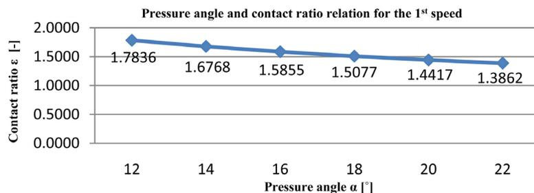
**Figure 14.** Contact ratio and pressure angle relation for the 1<sup>st</sup> speed.
