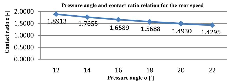
Figure 19. Contact ratio and pressure angle relation for the rear speed.
