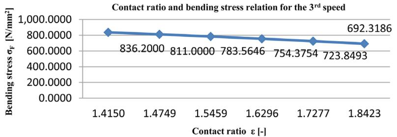
Figure 10. Contact ratio and bending stress relation for the 3<sup>rd</sup> speed.
