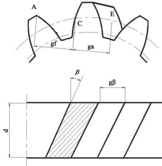
Figure 3. Contac line of helical gear.
