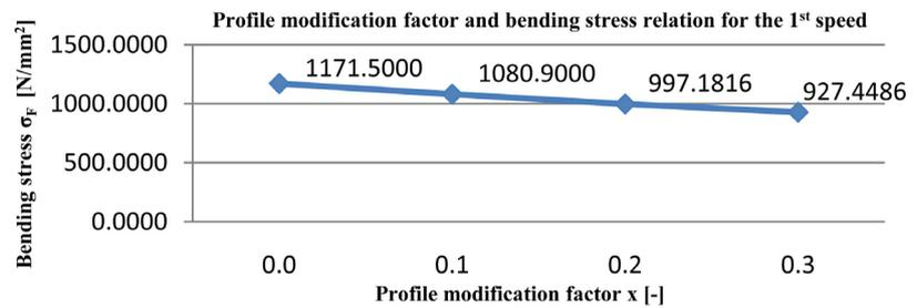
**Figure 20.** Profile modification factor and bending stress relation for the 1<sup>st</sup> speed.
