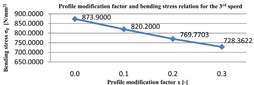
**Figure 22.** Profile modification factor and bending stress relation for the 3<sup>rd</sup> speed.
