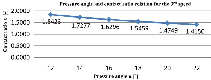
Figure 16. Contact ratio and pressure angle relation for the 3<sup>rd</sup> speed.
