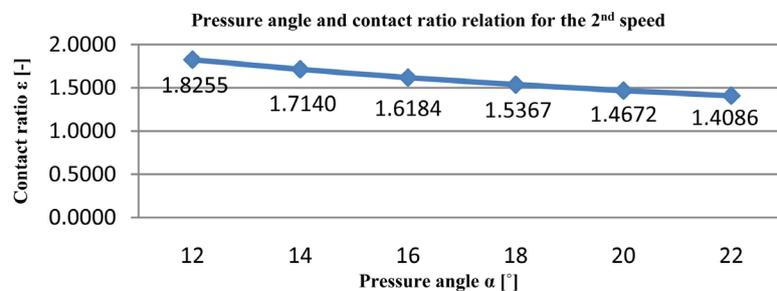
**Figure 15.** Contact ratio and pressure angle relation for the 2<sup>nd</sup> speed.
