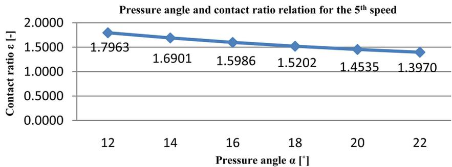
Figure 18. Contact ratio and pressure angle relation for the 5<sup>th</sup> speed.
