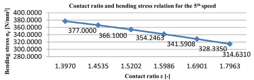
Figure 12. Contact ratio and bending stress relation for the 5<sup>th</sup> speed.
