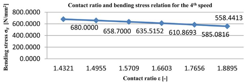
Figure 11. Contact ratio and bending stress relation for the 4<sup>th</sup> speed.
