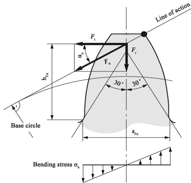
**Figure 5.** Bending stress at the tooth root.
