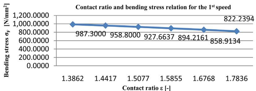
**Figure 8.** Contact ratio and bending stress relation for the 1<sup>st</sup> speed.
