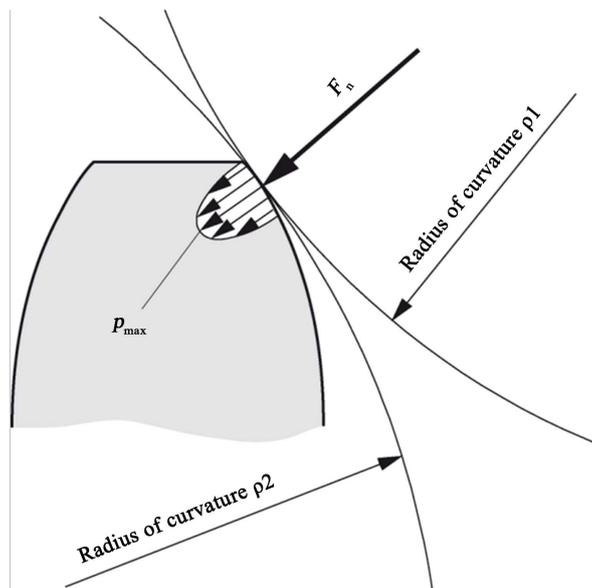
**Figure 6.** Contact stress at the tooth flank.
