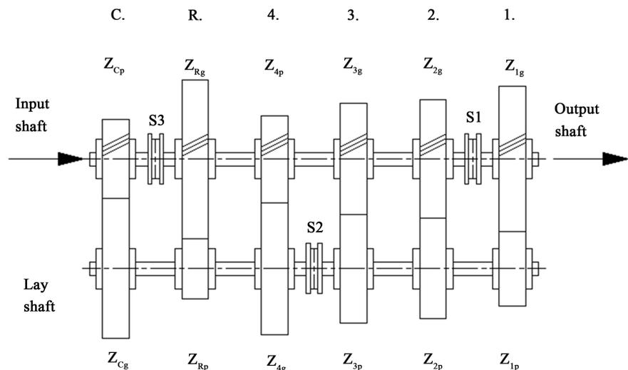
**Figure 1.** Five-Speed manual gearbox with helical gear for automotive transmission.
