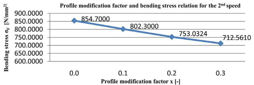
**Figure 21.** Profile modification factor and bending stress relation for the 2<sup>nd</sup> speed.
