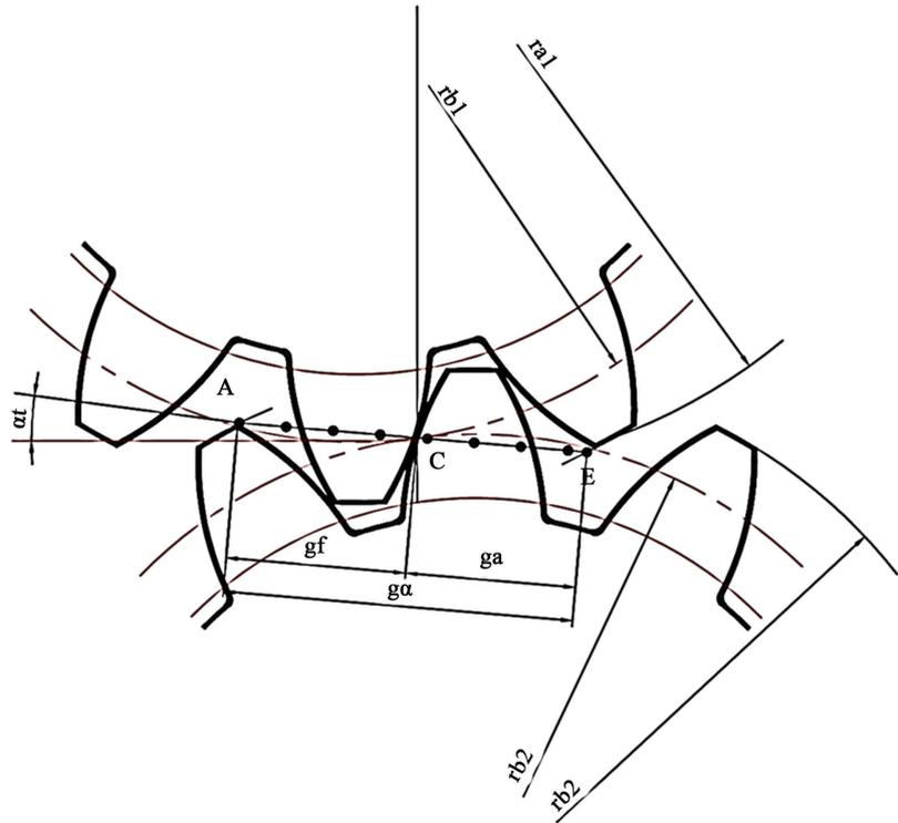
Figure 4. Contac line of helical gear including contact length AE.
