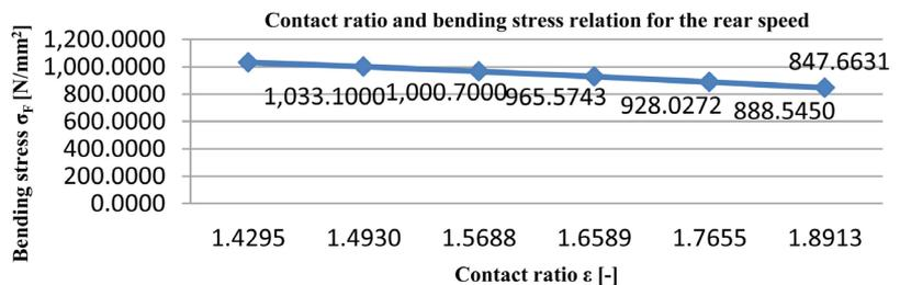
Figure 13. Contact ratio and bending stress relation for the rear speed.
