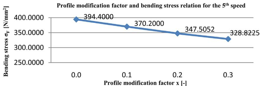
**Figure 24.** Profile modification factor and bending stress relation for the 5<sup>th</sup> speed.
