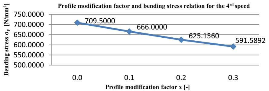
**Figure 23.** Profile modification factor and bending stress relation for the 4<sup>th</sup> speed.
