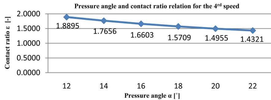
Figure 17. Contact ratio and pressure angle relation for the 4<sup>th</sup> speed.
