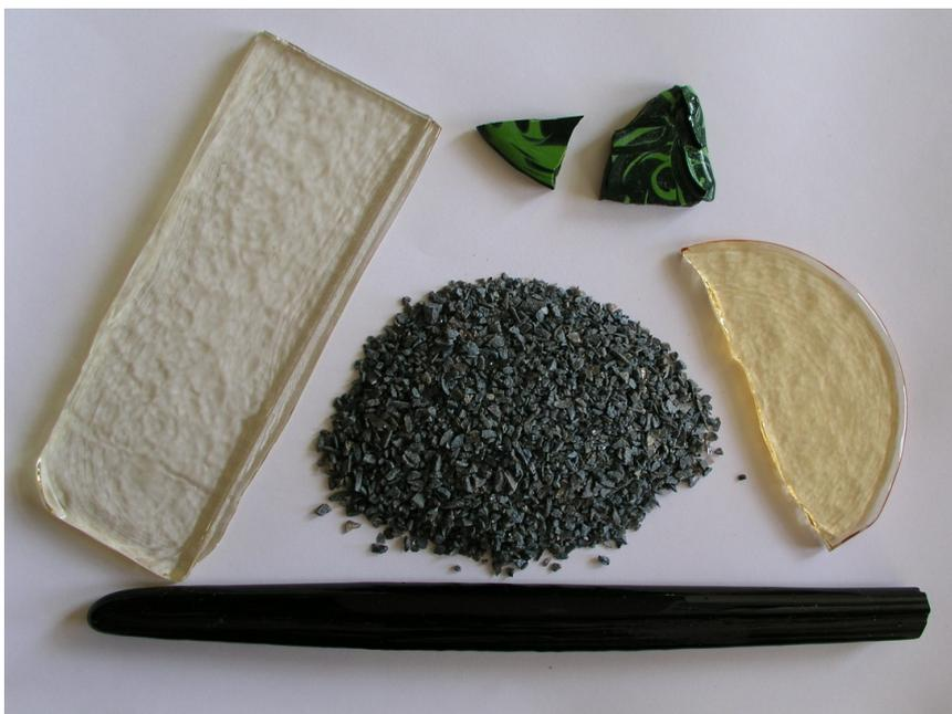
**Figure 11.** Appearance of glass based on furnace slags (slag is in the center).
