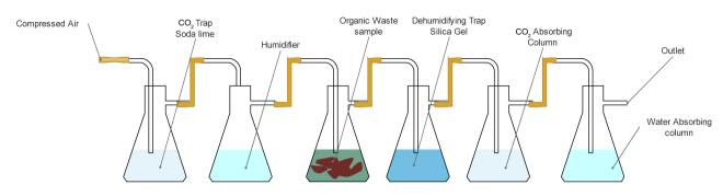
Figure 1. Set-up for determination of evolved carbon dioxide.
