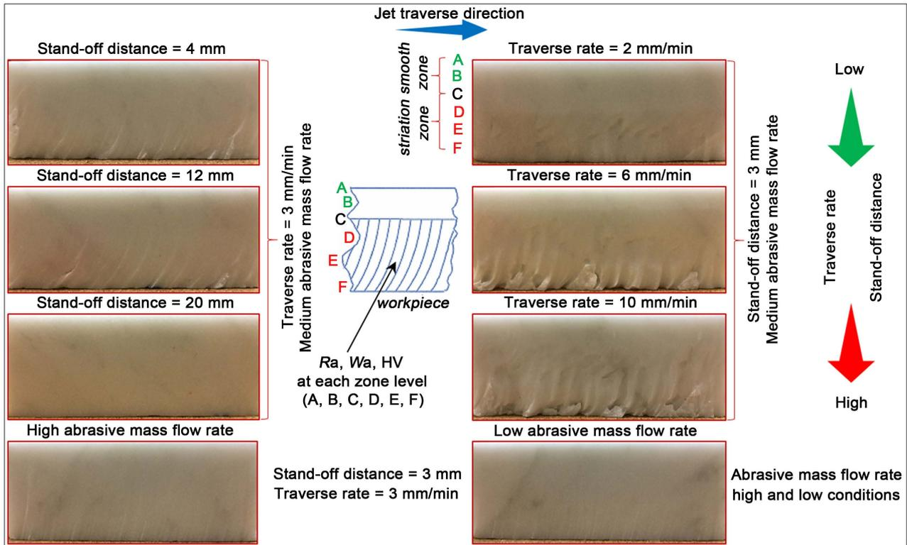
Figure 3. Illustration of AWJ cutting on Carrara marble.
