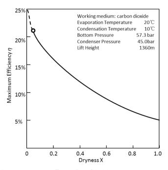
Figure 4. Maximum efficiency line of TGCC.
