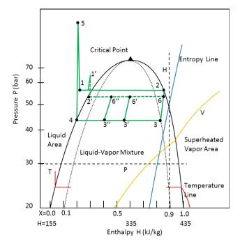
Figure 3. The P-H diagram of TGCC.
