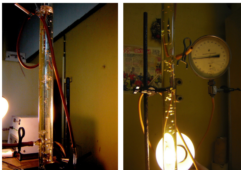
Figure 1. Laboratory rig for kerosene oxidation research.
