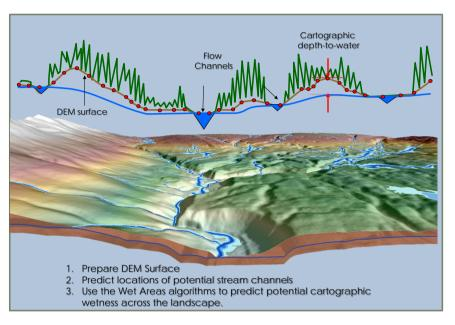
Figure 3. Flow channel and wet-areas mapping concept [2] [3].
