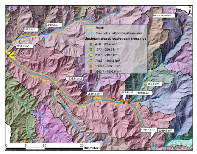
**Figure 7.** DEM-derived basin network with >4000 ha upstream basin areas for the upper component of the Choapa River watershed downslope from the Pelambres mine and east of Salamanca, with upslope watershed areas at each road-stream crossing.
