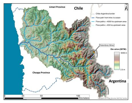
Figure 2. DEM-derived stream and river network of the Choapa River (Figure 1). Drainage pathways were derived from the Global 30 m SRTM DEM, hydro-conditioned with open street map (OSM) streams. Also shown: location of the open-pit mine at Los Pelambres.
