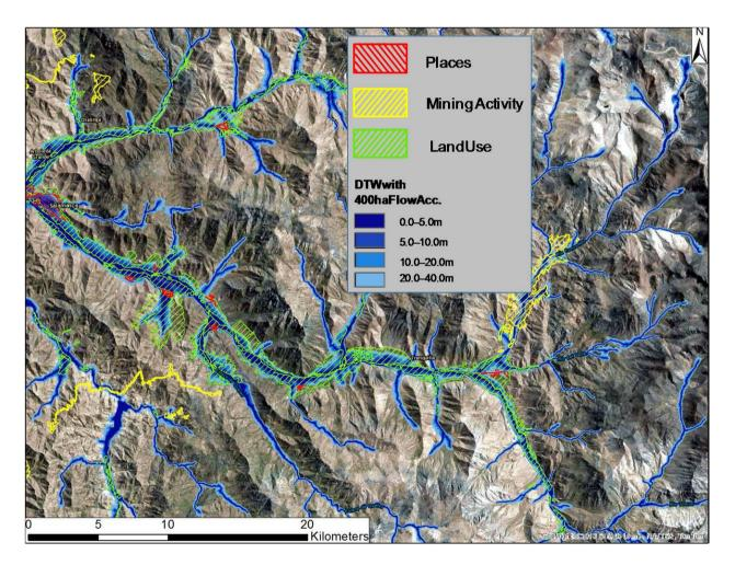
Figure 6. Overlaying the data layers for community locations, land-use pattern and mining activities over the DEM-derived cartographic depth-to-water index (DTW), ranging from 0 to 40 m (dark to light blue shading, respectively). Note the general conformance between 0 < DTW < 40 m and land-use extent along the major river valleys. Naturally occurring vegetation extends further upslope along streams, but becomes increasingly sparse further up along the slopes and flow channels.
