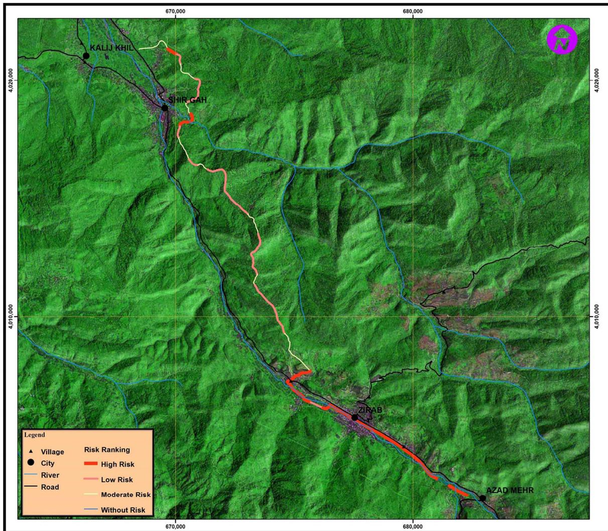
Figure 1. Pipeline placement position in the Satellite Image.
