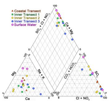
Figure 5. Piper diagram showing the water types and its proportions of Douala IV.
