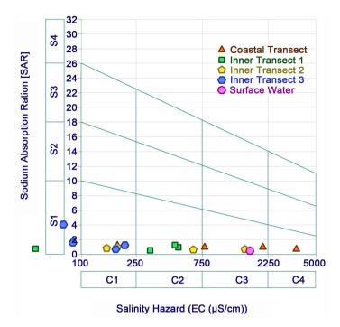
Figure 7. A classification of irrigation waters using the US Salinity diagram.
