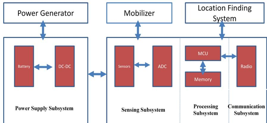
**Figure 2.** Architecture of a typical sensor node.
