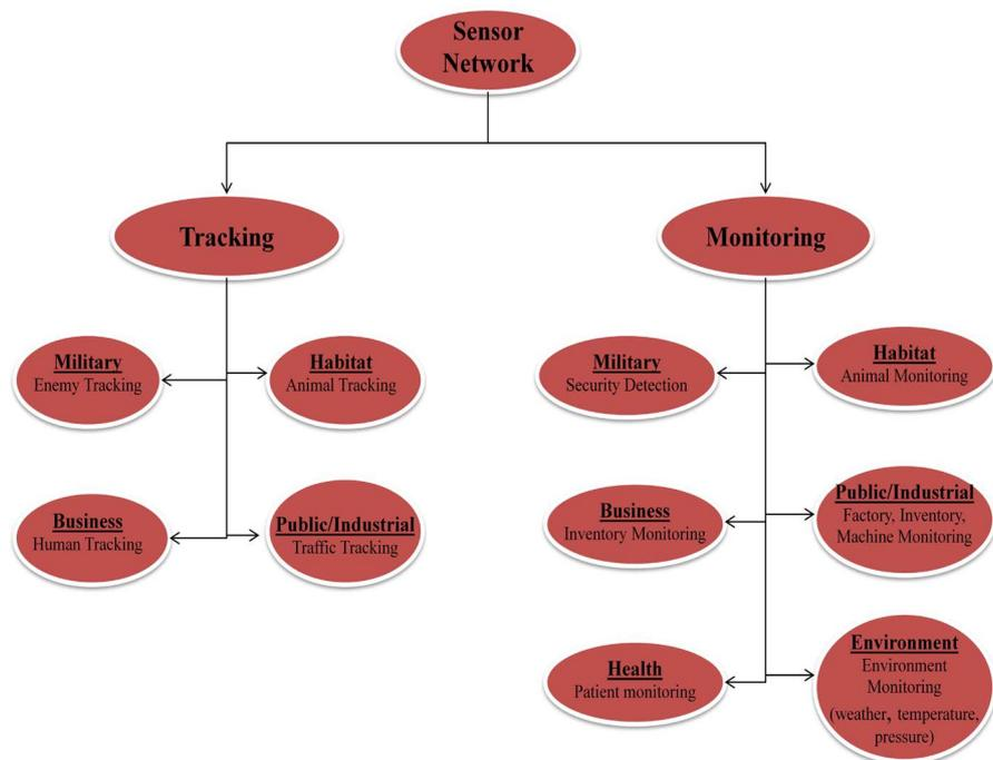
**Figure 4.** Overview of sensor network applications.
