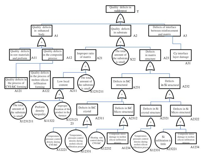
Figure 2. Fault tree of rudderpost quality.
