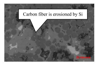
**Figure 4.** Metallographic scanning results of the rudderpost test specimens.
