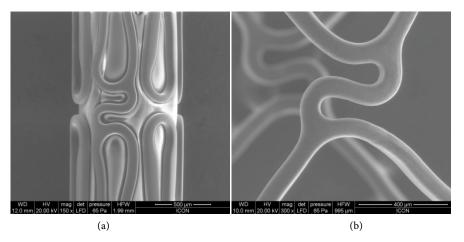
Figure 2. Scanning electron microscopy images of sterile (a) crimped stents and (b) expanded stents.
