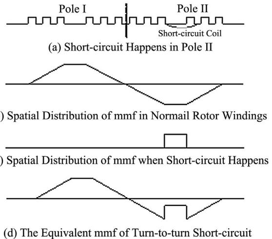
Figure 1. Spatial distribution of mmf in rotor windings
