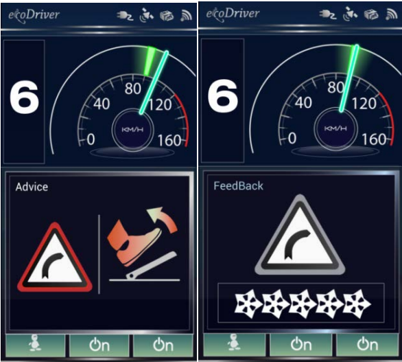
Figure 5. Advice and feedback when approaching a curve.
