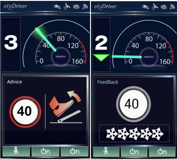
Figure 4. Advice and feedback when approaching a lower speed limit.
