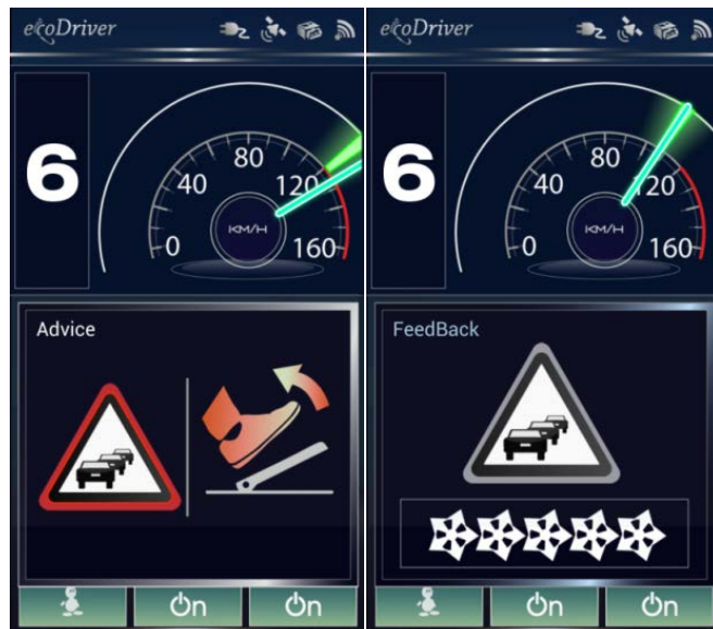
Figure 2. Advice and feedback for preceding vehicle detection.
