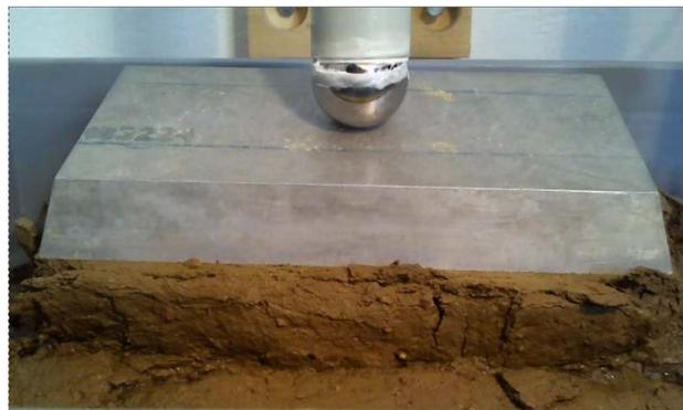
**Figure 1.** Wet adobe brick after fracture.
