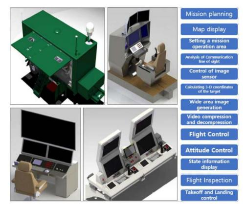
Figure 1. Representative features and various conceptual diagram for the ground control station
