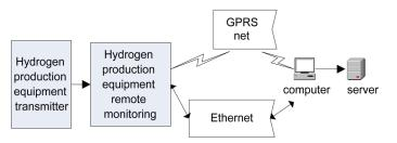
**Figure 1.** The framework of QDQ2-1 water electrolysis hydrogen production equipment monitoring system.
