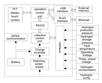
**Figure 2.** The structure of water electrolysis hydrogen production equipment remote monitoring terminal.
