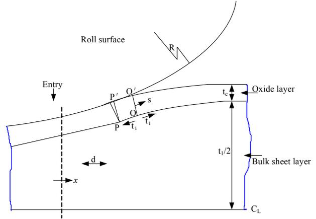
Figure 3. Schematic view for the crack initiation.
