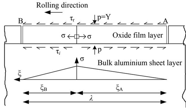
Figure 4. Model for roll bite oxide film fracture due to extension of the bulk metal.
