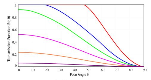
**Figure 6.** Alpha transmissivity  $E(r,\theta)/\pi a^2$ , Equation (49), in mica as a function of polar angle for different values of the radial coordinate (in cm) of the emission point: 2.0 (red), 1.0 (blue), 0.8 (green), 0.6 (violet), 0.4 (orange), 0.2 (plum).
