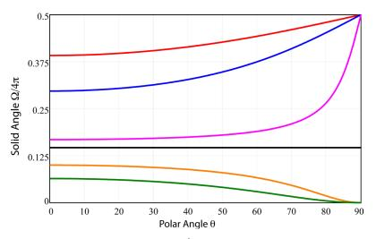
**Figure 3.** Fractional solid angle of detection  $\Omega/4\pi$ , Equation (46), as a function of polar angle for radial coordinates (in cm): 0.5 (red), 1.0 (blue), 2.0 (violet), a = 2.25 (black), 3.0 (orange), 4.0 (green).
