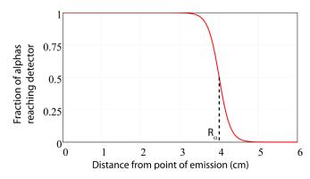
Figure 2. <sup>222</sup>Rn 5.5 MeV alpha particle range function (in air), Equation (41).
