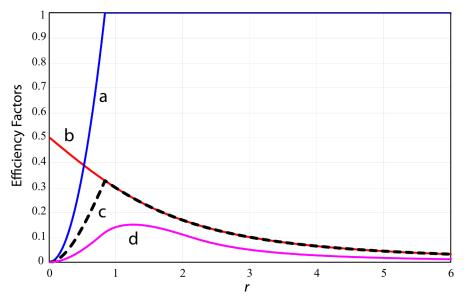
**Figure 7.** Radial dependence of factors contributing to detection efficiency of <sup>222</sup>Rn 5.5 MeV alpha emitted from a point source on the normal symmetry axis. (a) alpha transmissivity  $E(r,0)/\pi a^2$  in mica (blue); (b) solid angle  $\Omega(r,0)/4\pi$  (red); (c) efficiency
