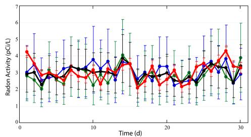
**Figure 8.** Sequence of 24-hour measurements of radon activity by GM method (red), commercial monitor COR1 (blue), commercial monitor COR2 (green), mean value ACOR of the two commercial monitors (black). The standard deviation of radon activity concentrations by (a) GM is approximately 0.32 pCi/L, (b) commercial monitor ranges from about 0.90 to 1.44.
