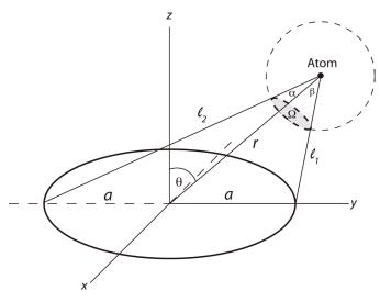
**Figure 1.** Azimuthally symmetric detection geometry. A radon atom located at coordinates  $(r, \theta)$  decays, producing an alpha particle that reaches the detector window of radius  $\alpha$  if emitted within solid angle  $\Omega$ .
