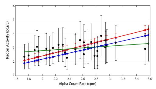
**Figure 9.** Plot of ACOR radon activity concentration (black) against corresponding GM alpha count rate. The three superposed lines show the GM activities based on Jacobi equilibrium (red) and secular equilibrium (blue), as well as the ML line of regression (green) to the ACOR points.
