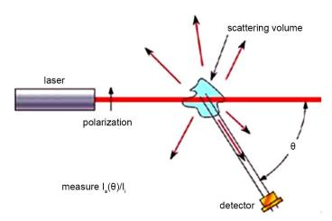
Figure 4. Typical light scattering experiment.
