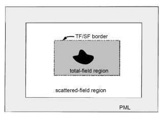
Figure 7. Schematic of total field/Scattered field description.
