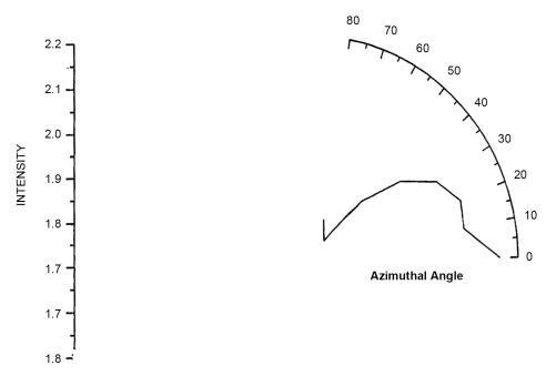
**Figure 23.** Scattered intensity vs azimuthal angle (at  $\theta$  = 30 for vert pol light).
