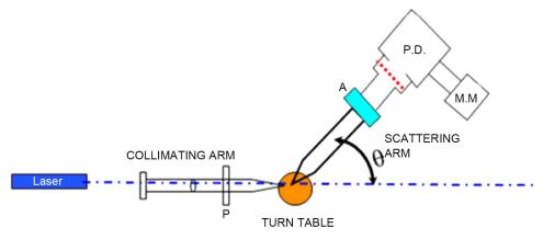
**Figure 8.** Experimental setup. P is polarizer, A = Analyzer, PD = Photo Diode, M.M. is the Multimeter.
