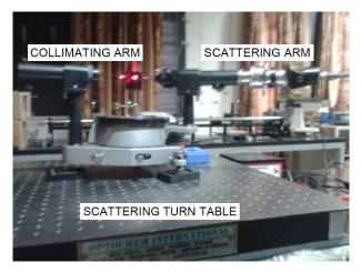
**Figure 9.** The fabricated Experimental Static Light Scattering setup. Collimating arm (with the polarizer), Scattering arm (with analyzer, Iris diaphragm, and Detector). The cell can be seen in the middle.
