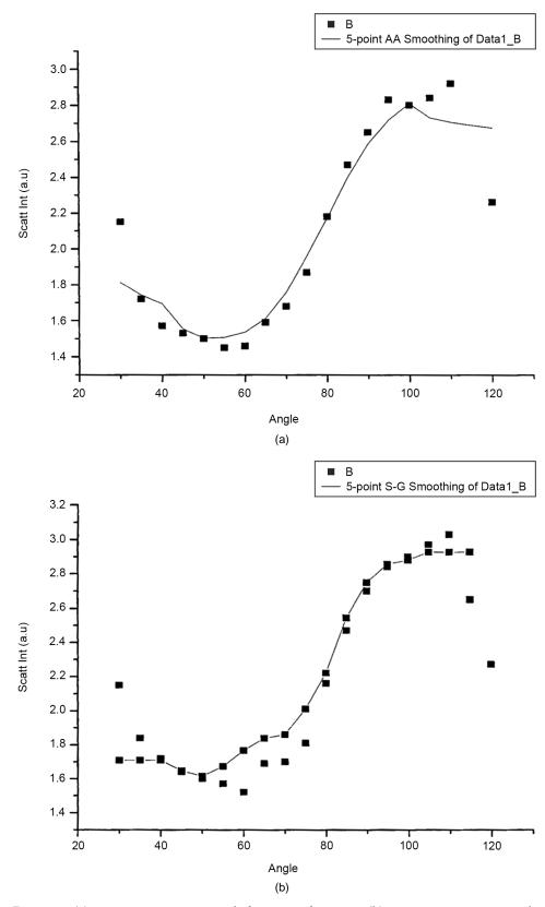
**Figure 14.** (a) Scattering intensity vs angle for CH configuration; (b) Scattering intensity vs angle for CV configuration.
