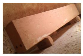
Figure 2. A view of a baked clay beam after firing in Potter's type kiln.
