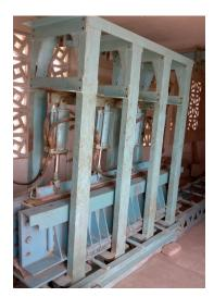
Figure 1. A clay beam is being cast and compacted in mechanized system.
