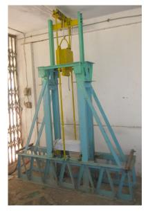
Figure 4. A reinforced baked clay beam of dimensions 150 mm  $\times$  150 mm  $\times$  500 mm is being tested for drop weight impact loading.
