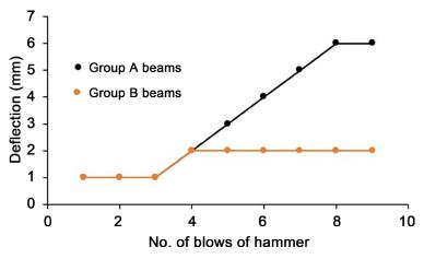
**Figure 5.** Impact load versus deflection response of RBC beams of group A (with two 12.7 mm diameter steel bars) and group B (with two 15.8 mm diameter steel bars).
