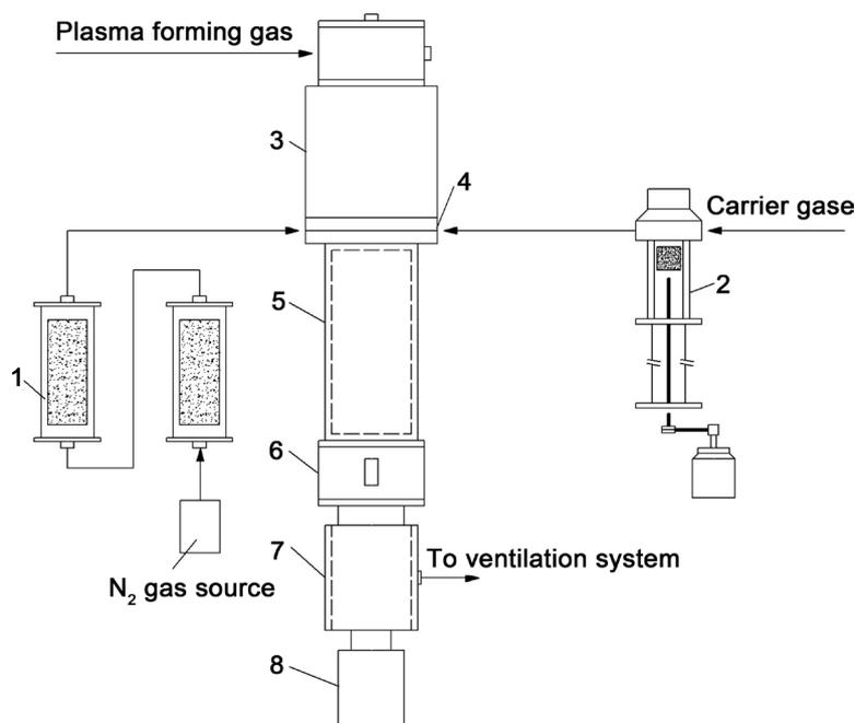
1—Gas purifying system; 2—Feeding equipment; 3—Plasmatron; 4—Reactant retractor; 5—Reactor chamber; 6—Heat exchanger; 7—Filter; 8—Powder collector
