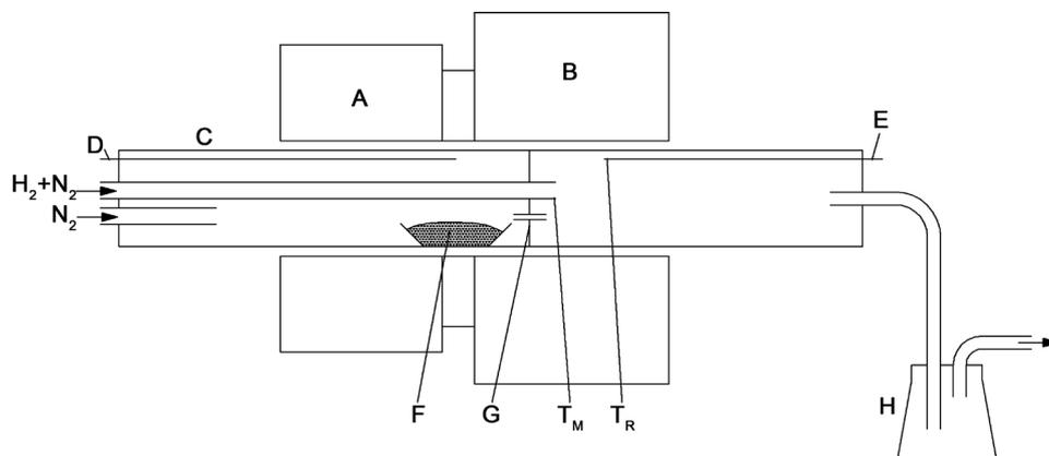
A, pre-heating furnace; B, main furnace; C, reaction tube; D, chromel-alumel thermocouple; E, Pt-Rh thermocouple; F, molybdenum boat; G, molybdenum plate and nozzle; H, flask
