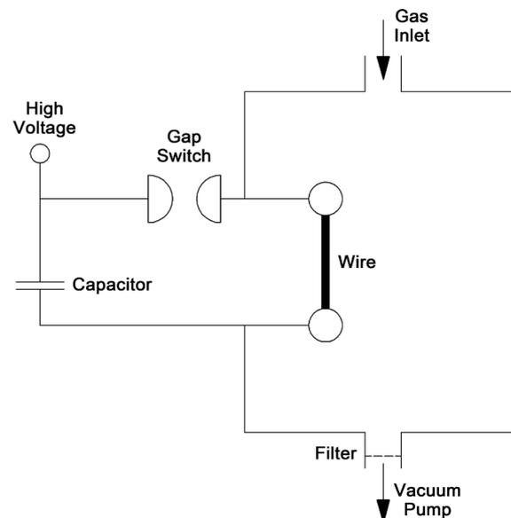
**Figure 1.** The schematic diagram of pulsed wire discharge technology.
