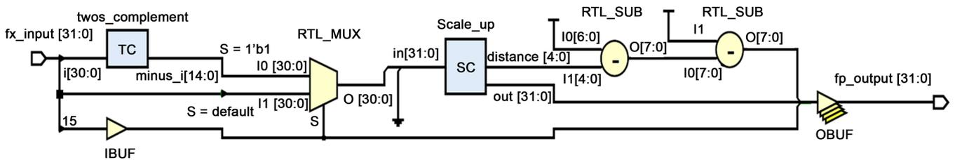
**Figure 13.** 32-Bit fixed-to-floating point FPGA schematic.
