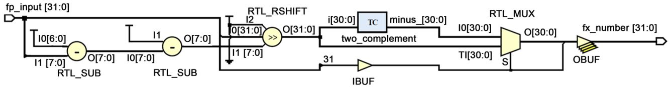
Figure 14. Floating to 32-bit fixed point FPGA schematic.
