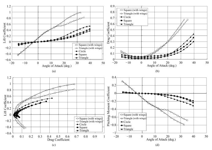
**Figure 4.** Aerodynamic characteristics of  $M_{\infty} = 0.9$ . (a) Lift coefficient; (b) Drag coefficient; (c) Polar curve; (d) Pitching moment coefficient.
