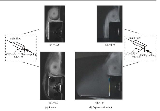
**Figure 8.** Smoke wire visualization result of "Square" and "Square with wings" at a = 30 deg.,  $U_{\infty} = 3$  m/s.
