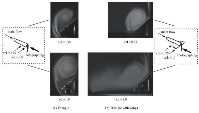
**Figure 9.** Smoke wire visualization result of "Triangle" and "Triangle with wings" at a = 30 deg.,  $U_{\infty} = 3$  m/s [17].
