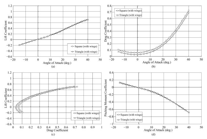
**Figure 5.** Aerodynamic characteristics of  $M_{\infty}$  = 4.0. (a) Lift coefficient; (b) Drag coefficient; (c) Polar curve; (d) Pitching moment coefficient.
