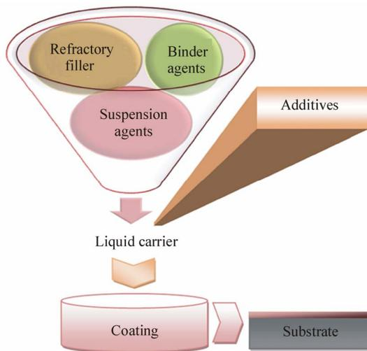
Figure 1. Coating components.
