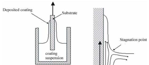
**Figure 5.** A schematic diagram of dip-coating process [35].
