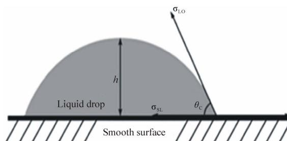
Figure 11. Shape of droplet on a smooth surface [57].
