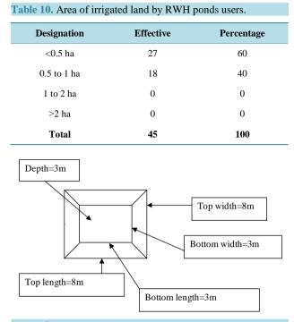
Figure 5. RWH pond geometry.
