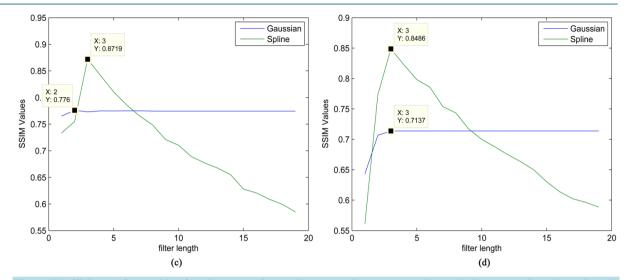
**Figure 4.** Efficiency of smoothing functions on various noise types using a  $7 \times 7$  edge mask size. (a) Motion Blur Noise; (b) Gaussian Noise; (c) Salt & Pepper Noise; (d) Speckle Noise.
