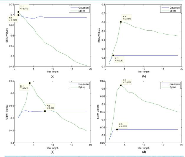
**Figure 2.** Efficiency of smoothing functions on various noise types using a  $3 \times 3$  edge mask size. (a) Motion Blur Noise; (b) Gaussian Noise; (c) Salt & Pepper Noise; (d) Speckle Noise.
