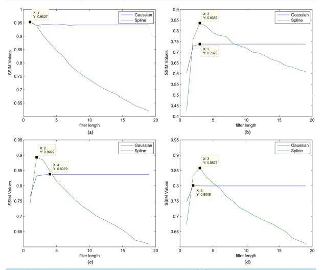
**Figure 5.** Efficiency of smoothing functions on various noise types using a  $9 \times 9$  edge mask size. (a) Motion Blur Noise; (b) Gaussian Noise; (c) Salt & Pepper Noise; (d) Speckle Noise.
