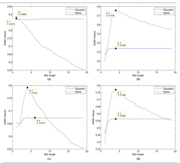
**Figure 3.** Efficiency of smoothing functions on various noise types using a  $5 \times 5$  edge mask size. (a) Motion Blur Noise; (b) Gaussian Noise; (c) Salt & Pepper Noise; (d) Speckle Noise.
