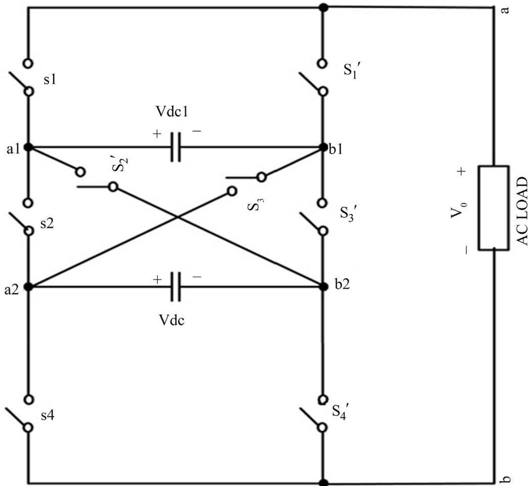
**Figure 2.** Proposed single phase nine-level inverter.
