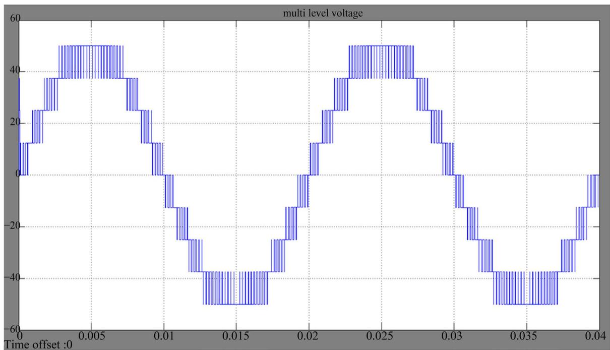
**Figure 12.** Single phase nine-level voltage output.
