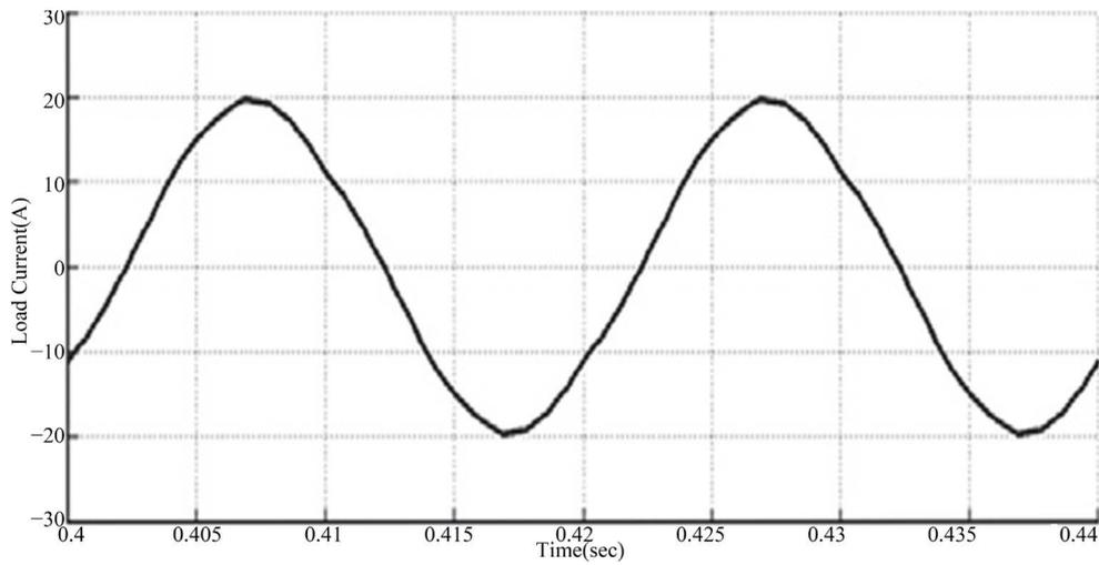
Figure 14. Load current waveform for nine-level voltage.
