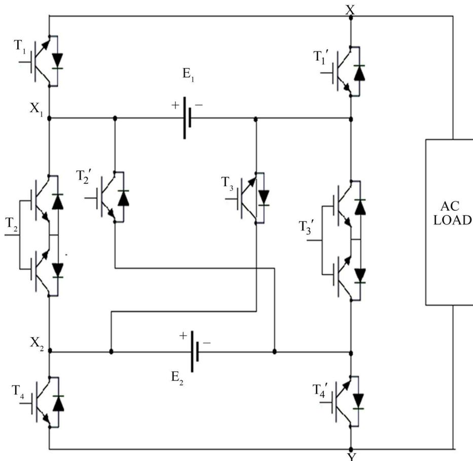
**Figure 3.** Proposed configuration for single phase nine-level inverter.
