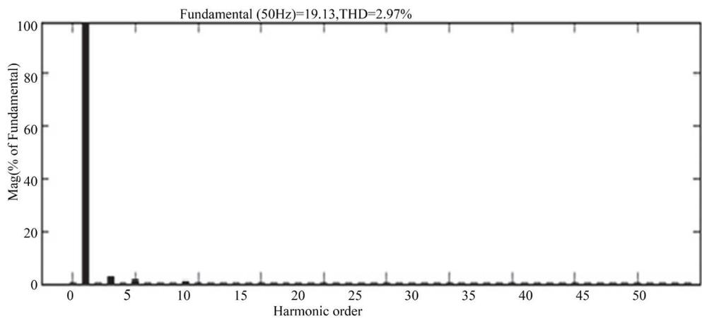
Figure 15. Harmonic spectrum for load current.
