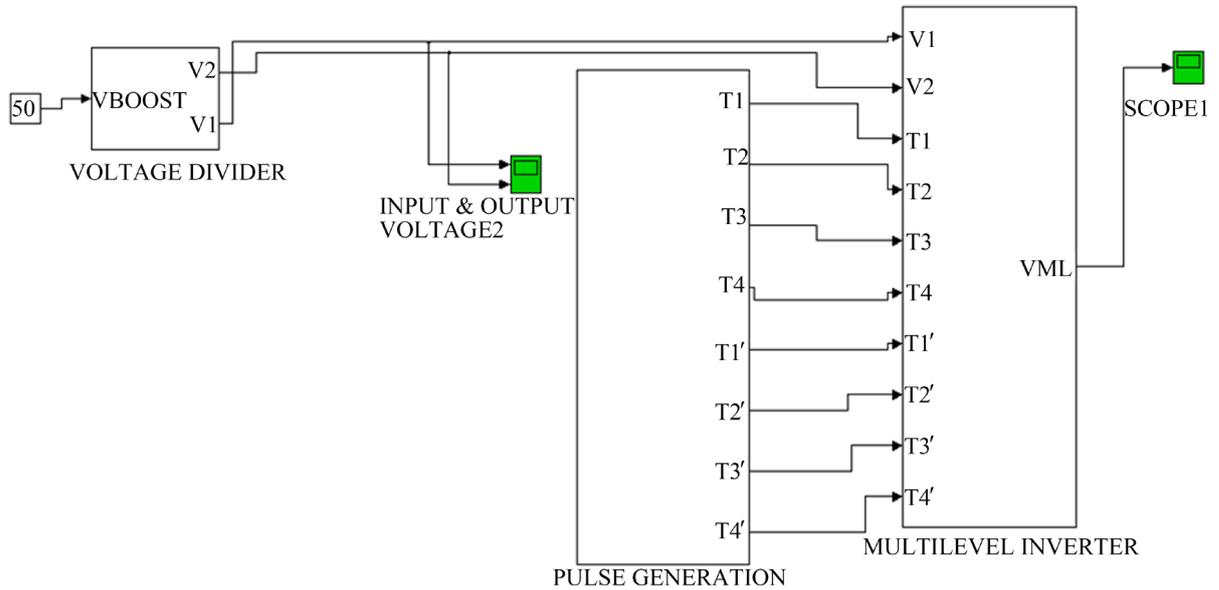
**Figure 11.** Overall simulation model for nine- level inverter.
