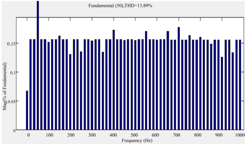
Figure 13. Harmonic spectrum of nine-level voltage output.
