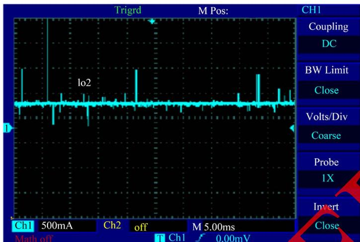
Figure 33. Start-up response of various input voltage ( $V_{in1} = 12\text{ V}$  and  $V_{in2} = 15\text{ V}$ ) and average output current of POEPCBC 2 [Ch1:500 mA/Div-load current].
