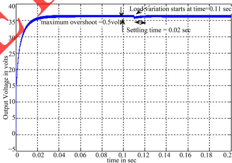
Figure 40. Output voltage of POEPCBC (50 Ω to 40 Ω).
