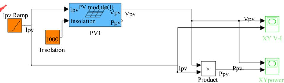
**Figure 2.** MATLAB model for single PV module.
