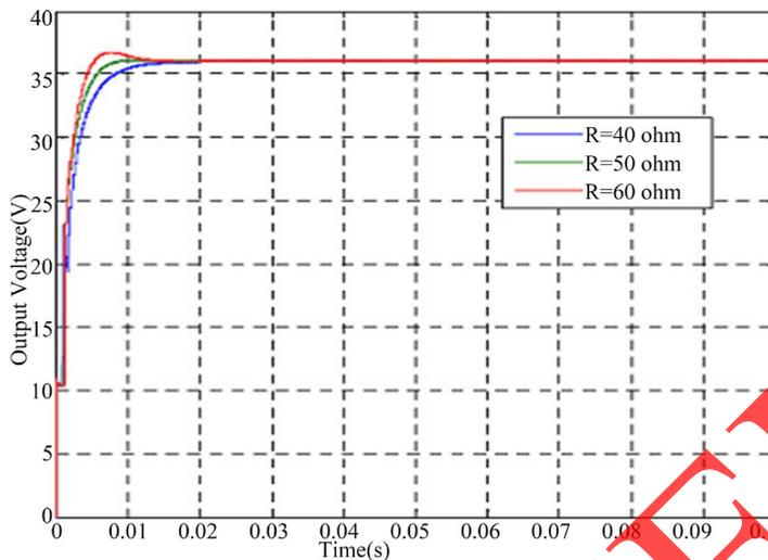
Figure 16. Response at start-up for output voltage of paralleled modules.
