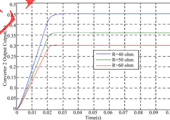
Figure 18. Response at start-up for average output current of POEPCBC 2.
