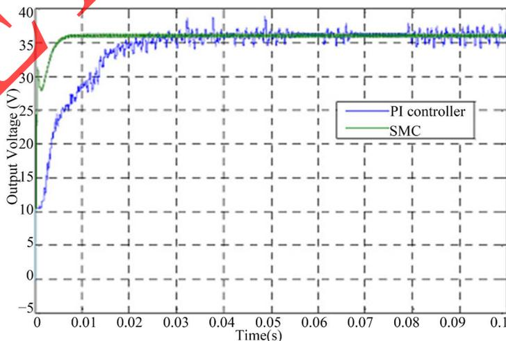
**Figure 26.** Performance of POEPCBC output voltage (100  $\mu\text{H}$  to 500  $\mu\text{H}$ ).
