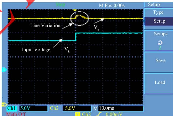
Figure 35. Output voltage of POEPCBC for input step change from 12 V to 15 V at time 0.05 s with  $R = 50\ \Omega$  [Ch1:5V/Div-output voltage and Ch2:5V/Div-input voltage].
