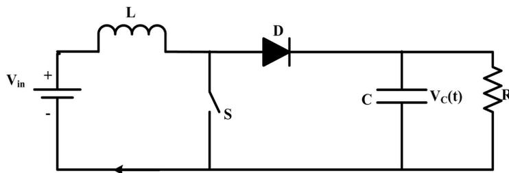
Figure 6. Equivalent circuit for the positive output elementary cascade boost converter.
