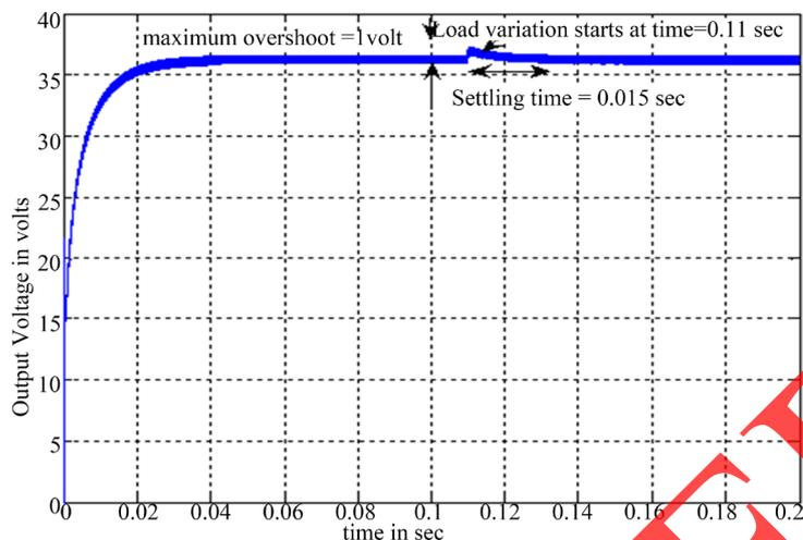
Figure 38. Output voltage of POEPCBC (50 Ω to 60 Ω).
