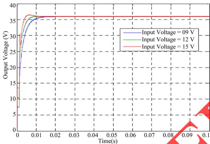
Figure 30. Start-up response of average output voltage of POEPCBC ( $R = 50 \Omega$ ).
