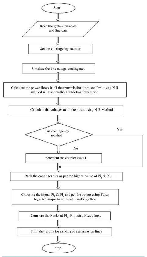
Figure 1. Flow chart for fuzzy logic implementation to contingency analysis.
