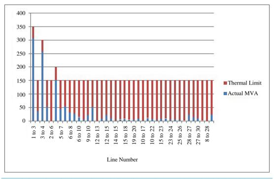
Figure 2. Comparison of real power flow in the lines after wheeling transaction against their thermal limit.
