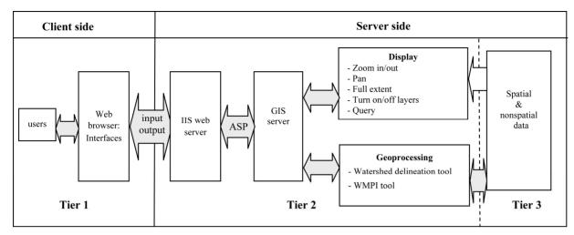
Figure 1. WebWMPI Architecture and transaction.
