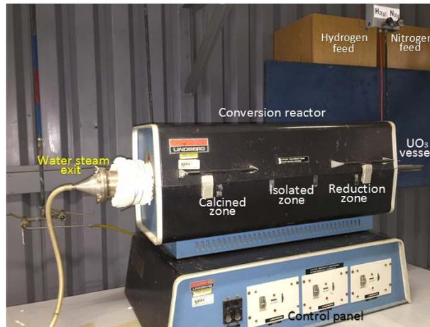
Figure 4. UO<sub>2</sub> conversion reactor.
