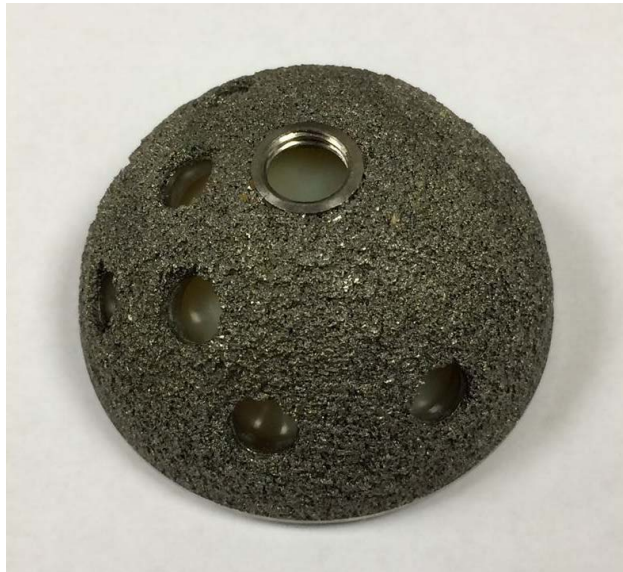
Figure 1. Rough porous surface of Regenerex Ring Loc+ cup with multiple screw holes.
