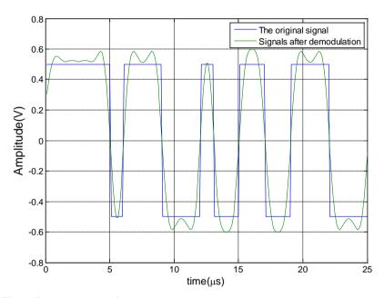
Figure 2. BPSK signals after demodulation.
