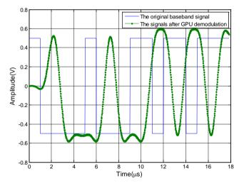
Figure 10. Signals after GPU demodulation.
