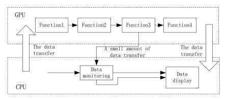
Figure 8. Parallel computing model of digital communication.
