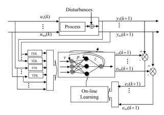
Figure 1. Principle of the neural modeling of the multivariable stochastic system.
