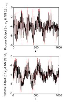
Figure 5. Output of process and NN of system (S2) using fixed learning rate.
