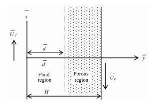
Figure 1. Physical configuration of the system.
