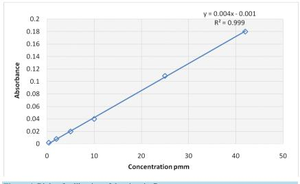
Figure 4. Right of calibration of the vitamin C.
