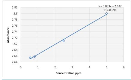
Figure 3. Right of calibration of the vitamin B.
