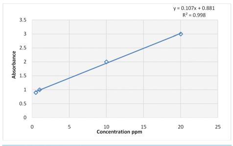
Figure 6. Right of calibration of iron.
