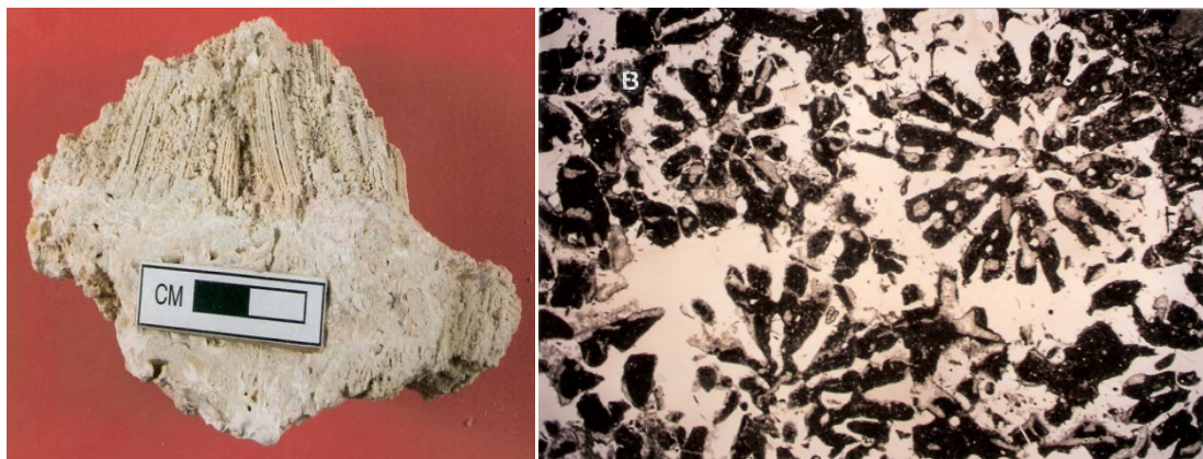
Figure 9. (A) Tarbellastraea sp. from Benghazi Formation at Benghazi (Al Hawari) Cement Quarry, (B) Thin section from the same colony shows mouldic porosity (in black). Field of view = 6 mm, (XPL).
