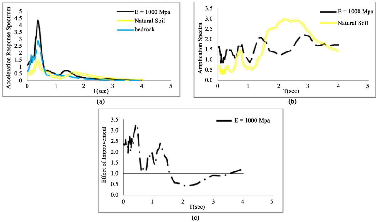
**Figure 15.** Comparison of seismic response on the surface of the natural ground and its improvement under near-fault Loma Prieta earthquake with PGA = 0.7 g: (a) elastic response spectra, (b) amplification of Sa, (c) the effect of improvement on Sa.
