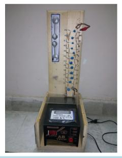
Figure 1. High voltage lightning impulse generator.
