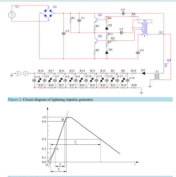
Figure 3. Standard impulse waveform [5].
