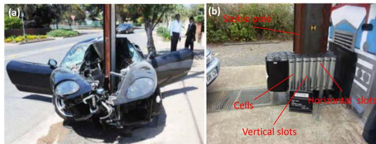
**Figure 1.** (a) Collision with fixed object (e.g. Stobie pole) [5]; (b) hollow tube based buffer system installed around Stobie pole [29].
