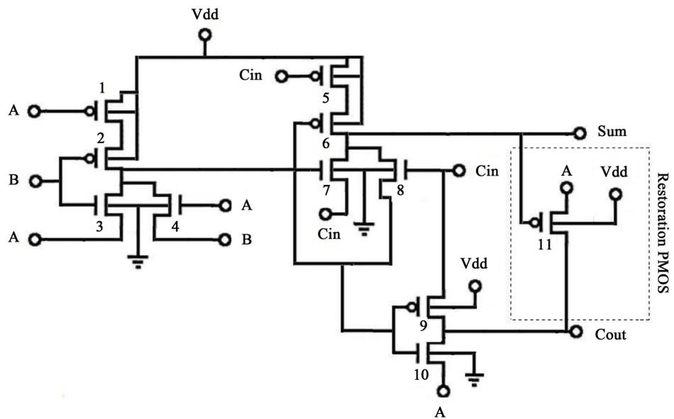
Figure 9. The proposed adder cell.
