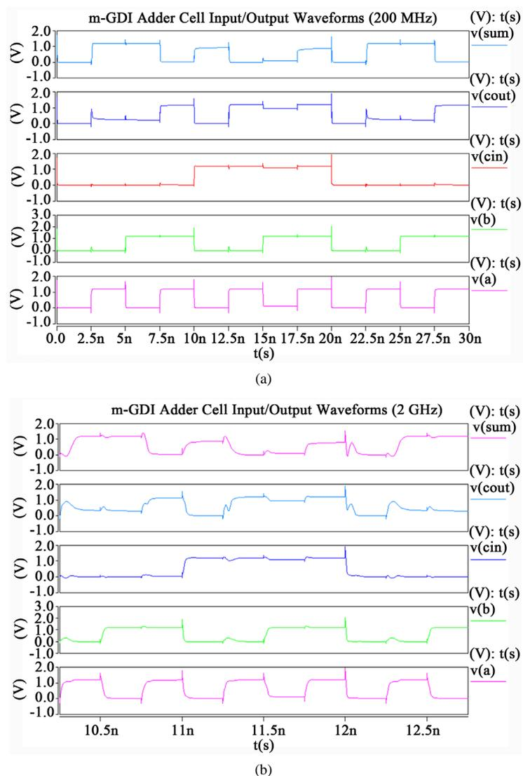
**Figure 12.** The m-GDI adder cell input/output waveforms in 90 nm technology (a) 200 MHz; (b) 2 GHz.
