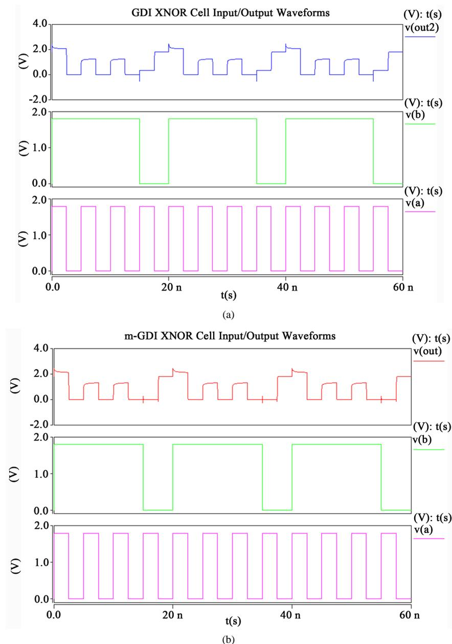
**Figure 10.** The input/output waveforms of XNOR cells (a) GDI; (b) m-GDI.
