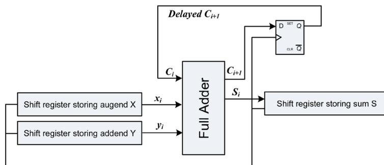
**Figure 1.** A serial adder.
