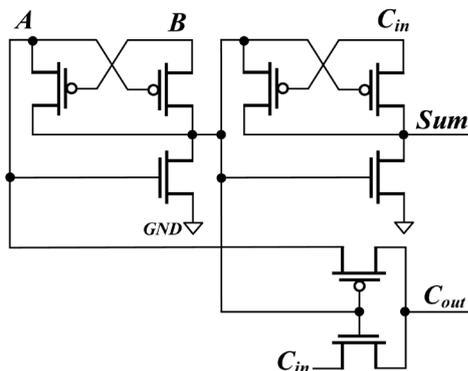
Figure 4. The 8 transistors full adder.
