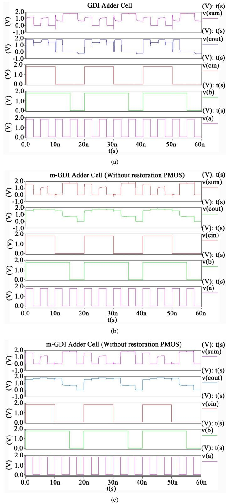
**Figure 11.** The input/output waveforms of adder cells (a) GDI XNOR full adder; (b) m-GDI XNOR full adder, without restoration PMOS; (c) m-GDI XNOR full adder, with restoration PMOS.
