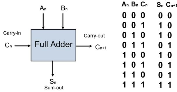
**Figure 2.** The logic symbol and truth table for a full adder.
