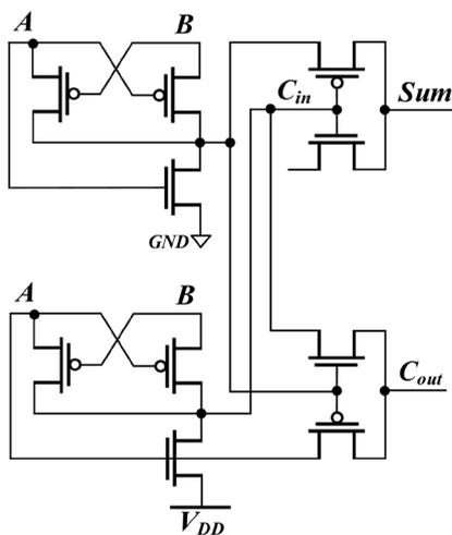
Figure 5. The 10 transistors full adder.
