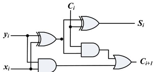
Figure 3. The logic network for a full adder.
