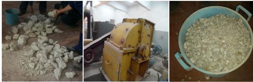
**Figure 2.** Different phases for preparing recycled, crushing and sieved CDW.
