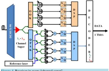
Figure 4. Receiver in every "channel super".
